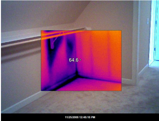
Purple area shows missing or inadequate insulation in master bedroom closet knee-walls.
