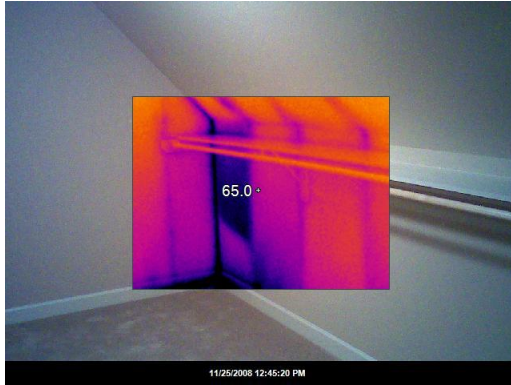
Purple area shows missing or inadequate insulation in master bedroom closet knee-walls.
